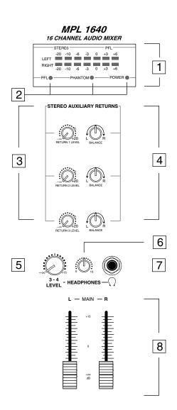
**1: Meter** - This seven-segment bar meter shows the continuous output level of the Main L/R stereo output. For optimum signal-to-noise ratio, try to adjust all levels so that program material is usually at or around 0 VU, with occasional but not steady excursions to the red +3 or +6 segments. See the "Setting the Correct Gain Structure" section on page 12 for more information.
